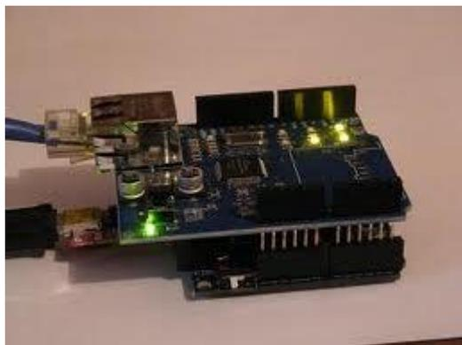
**Figura 2. Arduino com *Shield Ethernet***
